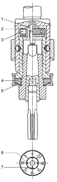
If, for example, you want to cut a thread M12 in steel 70-2 with tapping adaptor GE34-MT3, the setting for this according to the table on page 3 is IV/12. IV refers to the position of the built-in cup springs (5) and 12 is the setting number on the adjusting nut (2).
